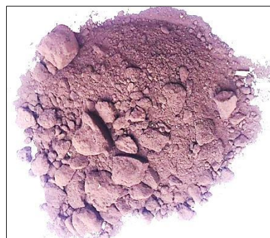
Fig. 8 Appearance of Nsuta Pyrolusite Ore after 60 min Calcination in the Presence of PS
