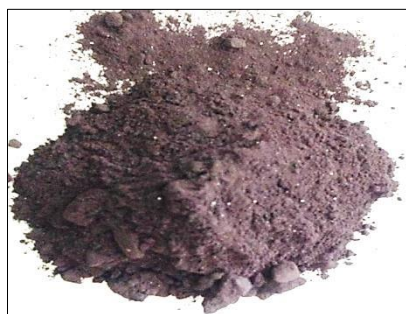
Fig. 7 Appearance of Nsuta Pyrolusite Ore after 60 min Calcination in the Absence of PS
