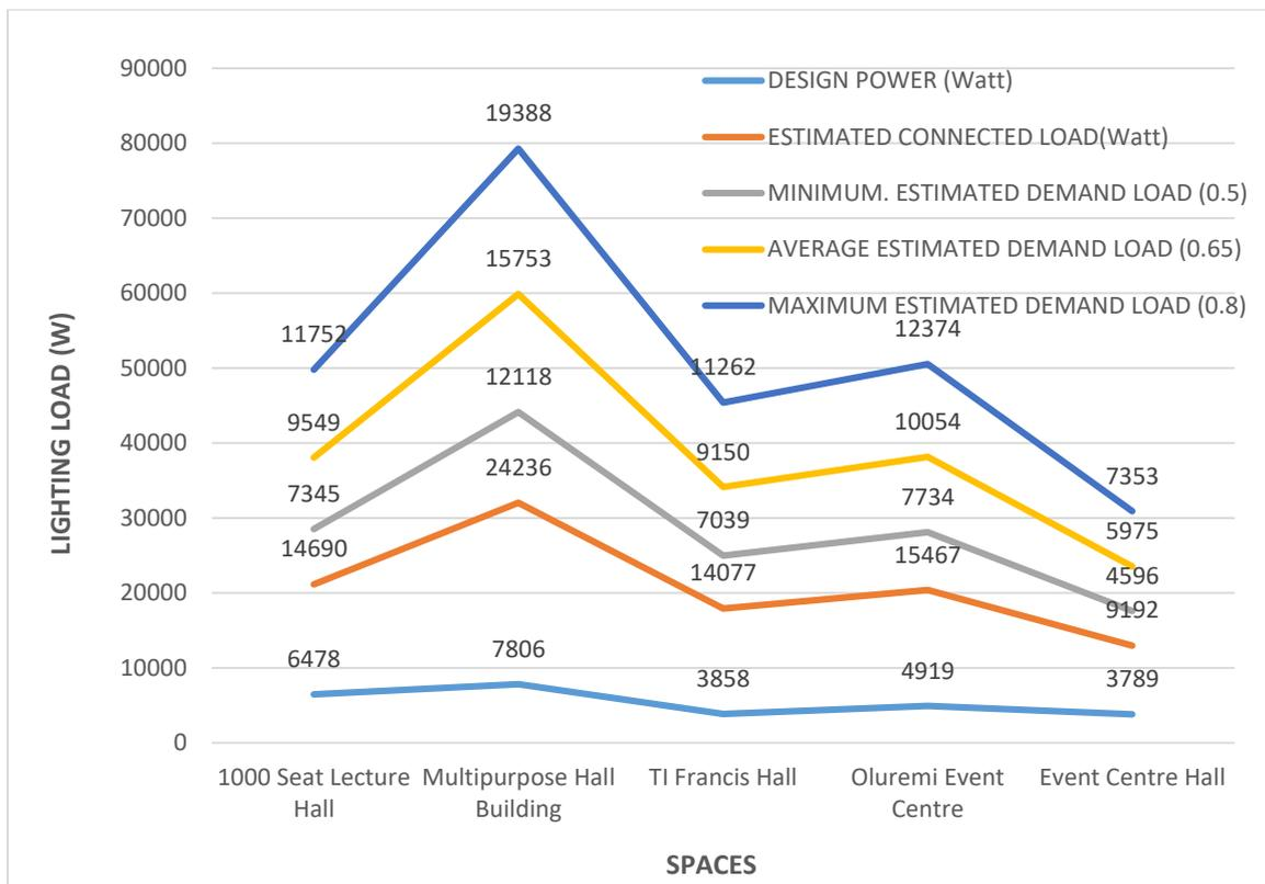
**Figure 2 Design Load versus Estimations**
