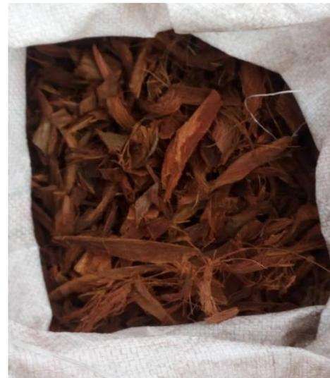
**Fig. 2 Coconut Husk Cut into Pieces for Milling**
