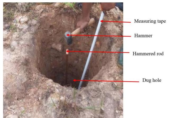
**Fig. 7 Hammered Rod in the Dug Hole**
