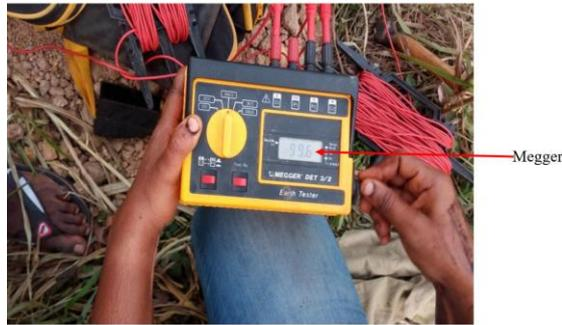
**Fig. 8 Megger Used for the Resistance Readings**
