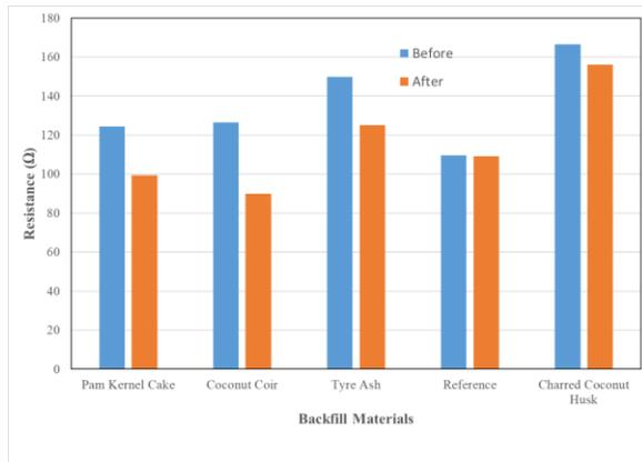
**Fig. 10 Graph of the Resistance Values before and after Backfilling**
