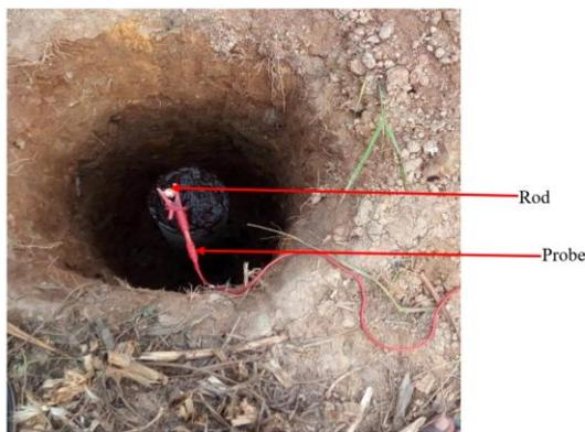
**Fig. 9 Probe Attached to the Rod for Resistance Readings**
