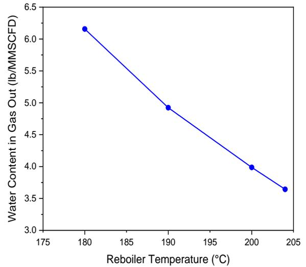
**Figure 6 Outlet Gas Water Content against Reboiler Temperature at 8 Contactor Stages and TEG Flow Rate of 1m<sup>3</sup>/hr**
