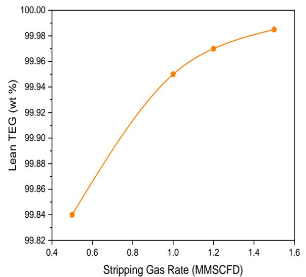
**Figure 7 Lean TEG against Stripping Gas Flow Rate**
