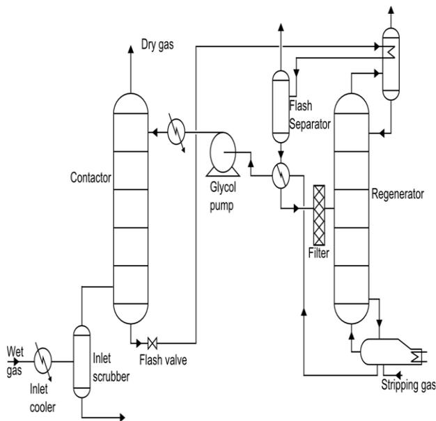
**Figure 2 Typical Glycol Dehydration Process**
