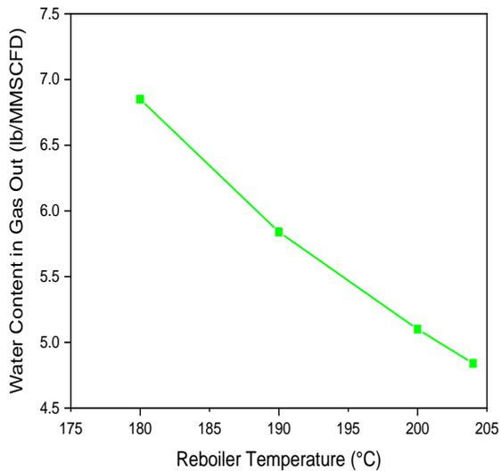
**Figure 5 Outlet Gas Water Content against Reboiler Temperature at 8 Contactor Stages and TEG Flow Rate of 0.5 m<sup>3</sup>/hr**
