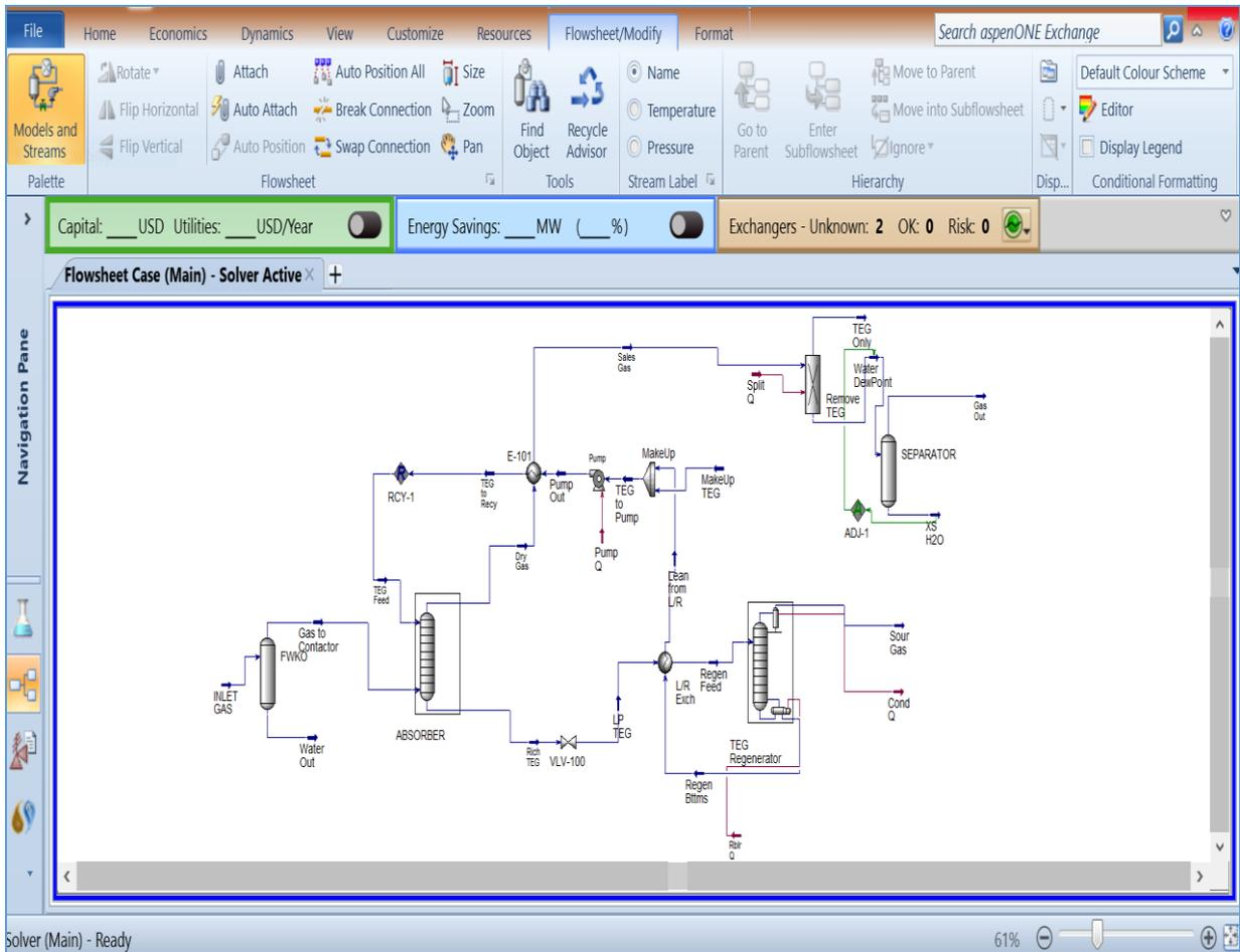
Figure 4 Complete Process Flow Diagram
