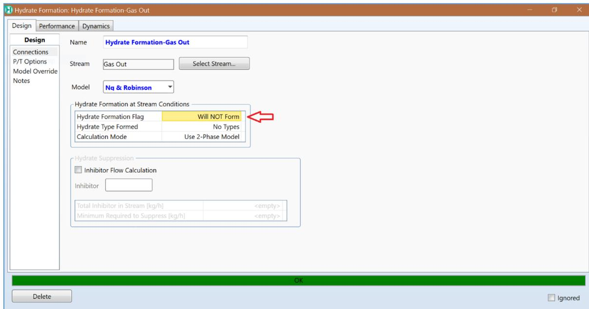
**Figure 8 Hydrate Formation Possibility of Gas Outlet Stream**
