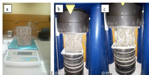
Figure 5: (a) Weighed Cube (b) Concrete Cube under Compressive Machine (c) Crushed Concrete Cube under Compressive Machine
