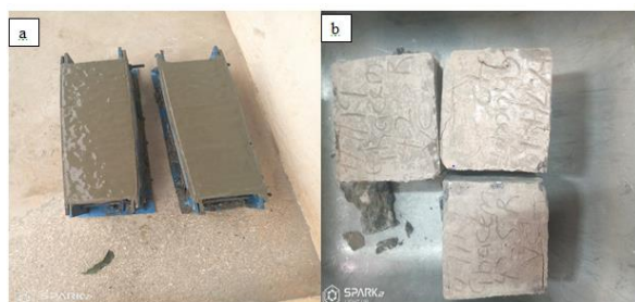
Figure 4: (a) Casted Concrete Cubes (b) Dried Concrete Cube
