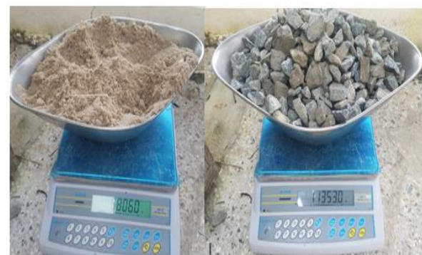
Figure 2: (a) Fine Aggregate (b) 19 mm Coarse Aggregate
