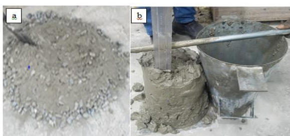
Figure 3: (a) Mixed cements and Aggregates (b) Slump test
