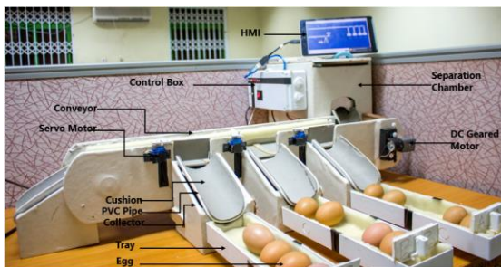
Fig. 7 Egg Collection and Sorting Machine Operation
