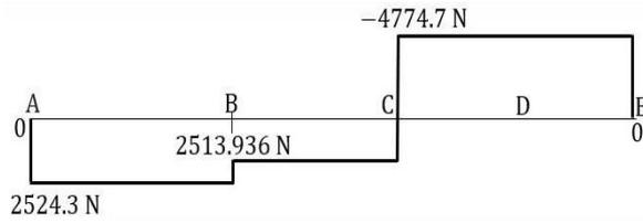
**Fig. 10 Shear Force Diagram for Horizontal Loading**
