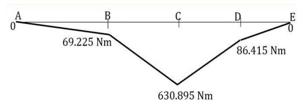
**Fig. 8 Bending Moment Diagram for Vertical Loading**
