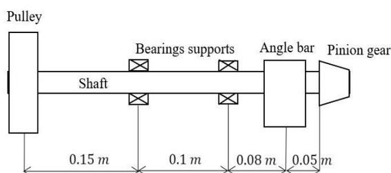
**Fig. 5 Shaft Geometry and Loads**
