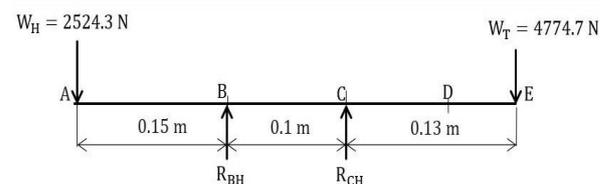
**Fig. 9 Space Diagram for Horizontal Loading**
