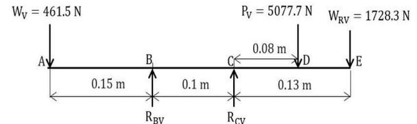
**Fig. 6 Space Diagram for Vertical Loading**
