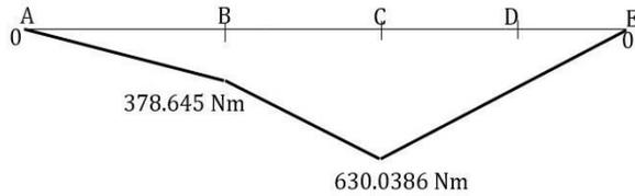
**Fig. 11: Bending Moment Diagram for Horizontal Loading**
