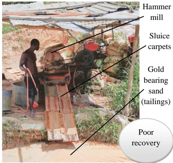
**Fig. 1 Setup of a Hammer Mill and a Traditional Sluice System**
