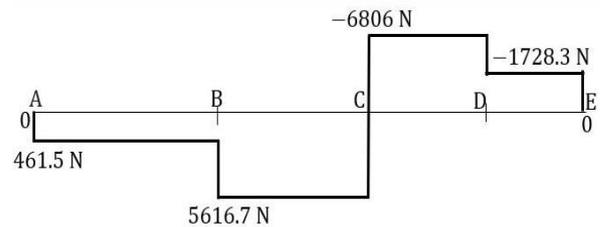
**Fig. 7 Shear Force Diagram for Vertical Loading**
