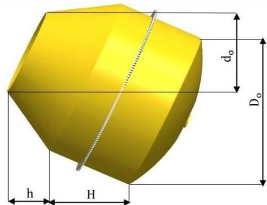
Fig. 4 Dimensions of the Drum
