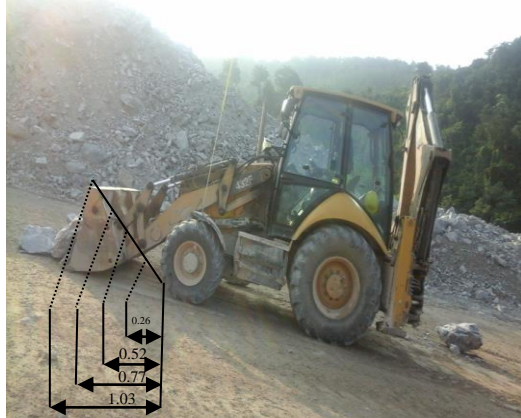
Fig. 1 Direct Observation and Measurement ( m^3 ) with CAT 432F Backhoe
