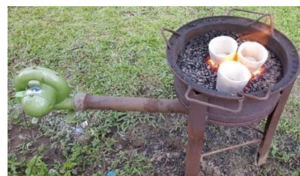
Fig. 3 Custom-made Furnace consisting of End-of-life Vehicle Tyre Rim and a Blower Assembly
