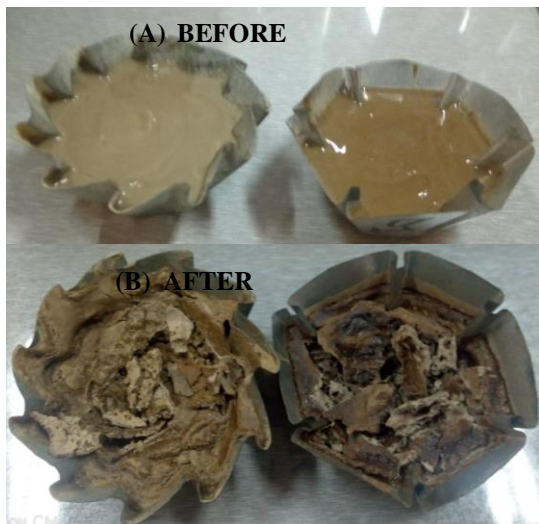
Fig. 2 Mud Samples showing ENV and INV Mud: (A) before Drying and (B) after Drying
