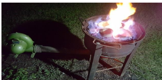
Fig. 3 Firing of Crucibles containing End-of-life Toner Powder.
