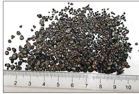
Fig. 15 Samples of Metallic Iron Produced from Heating Composite Pellet of Pudo Iron Ore with Waste Toner Powder
