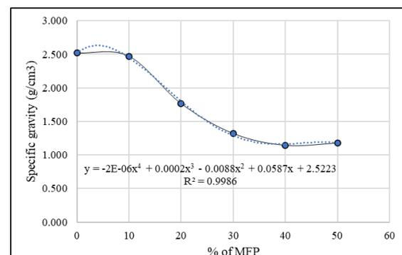
**Fig. 3. A Correlation Between Specific Gravity and % of MFP**
