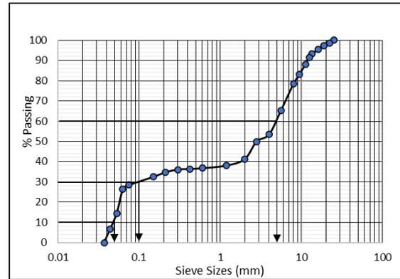
**Fig. 4. Grading Curve for Laterite**
