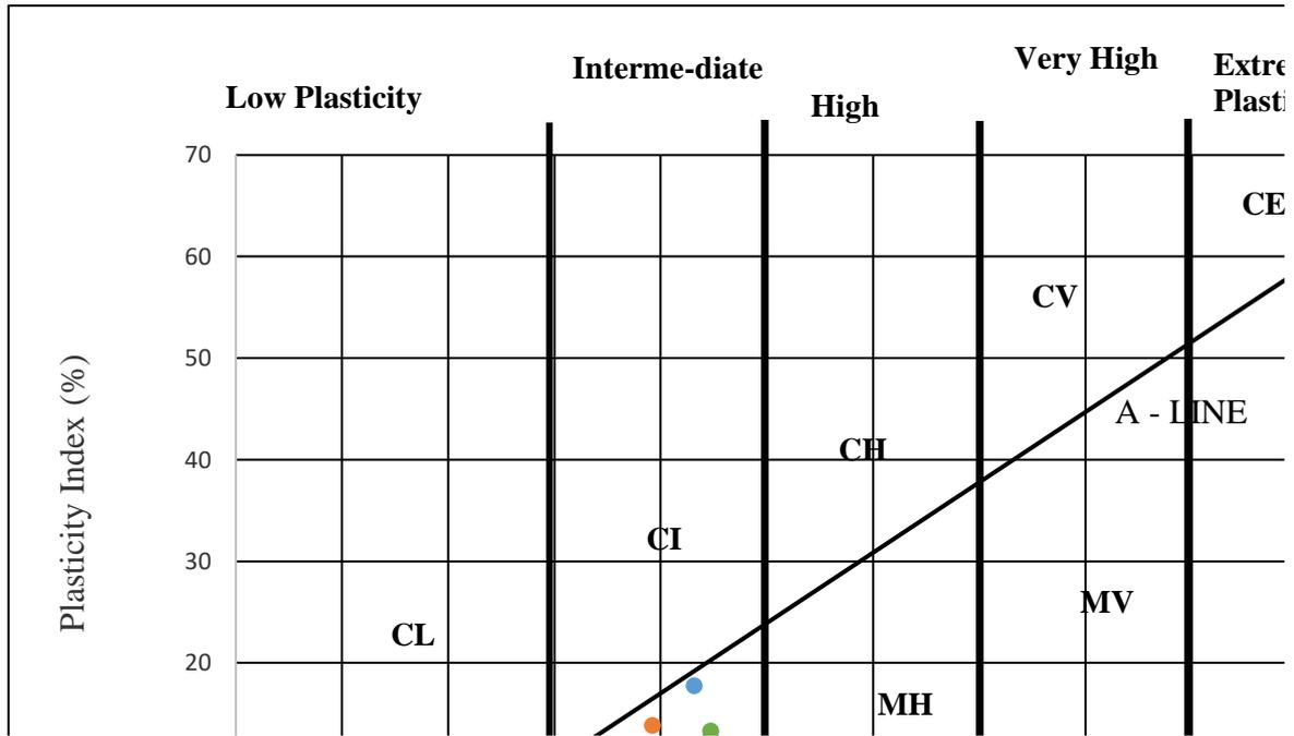
Fig. 6. Plasticity Classification for Lateritic Soil with Respect to their %MFP
