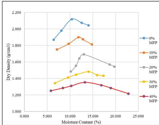
Fig. 7. Compaction Characteristic Curves
