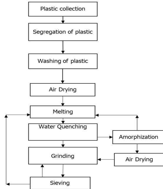
**Fig. 2. Plastic Waste Collection and Preparation Process**
