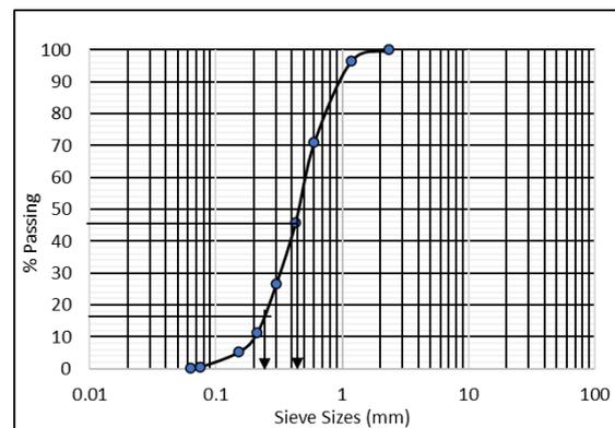
**Fig. 5. Grading Curve of 100 % MFP**
