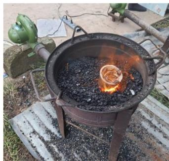
**Fig. 2 Firing of Crucibles containing Samples**
