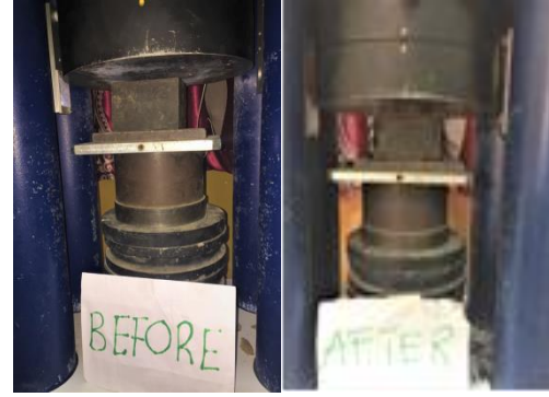
Figure 8 Compressive Strength test.
