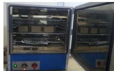
Figure 6 MW oven for firing of bricks
