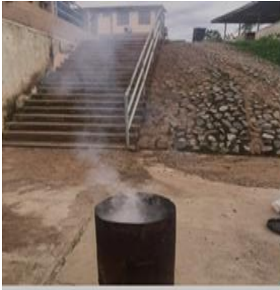
Figure 3.3 Conventional Method of Carbonization Showing Smoke Emission
