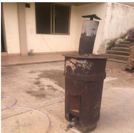
Figure 3.4 Smokeless Charring in the Down Draught Pyrolysis Reactor
