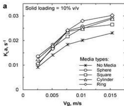
**Fig. 1** Overall mass transfer coefficient ( $K_{La}$ ) in bubble column reactor of each solid media type with: (a) superficial gas velocity ( $V_g$ ) and (b) solid loading (Sastaravet *et al.*, 2020)
