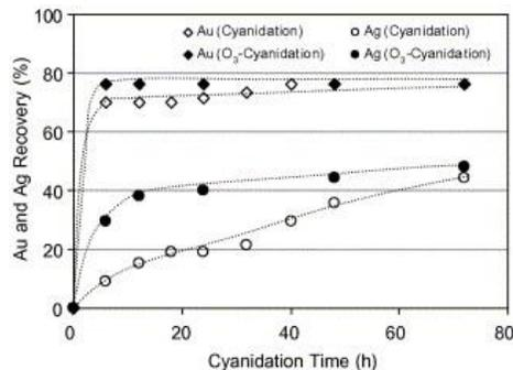
**Figure 5** Gold and silver recoveries of mineral A when treated by direct ozone addition and cyanidation. (Elorza-Rodríguez *et al.*, 2006)
