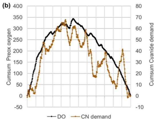
**Figure 3** Reactivity number or oxygen demand survey plots for the concentrate pre-oxidation circuit (September – October 2017).
