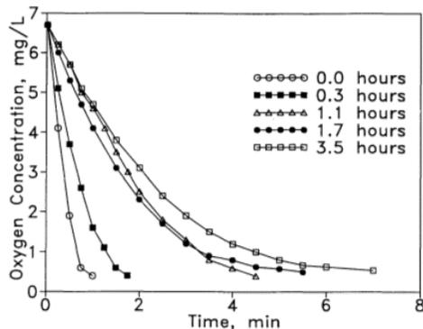
**Figure 9** Rate of Oxygen removal from sample pulp as a function of aeration time during Filblast unit test (Bodnaras *et al.*, 1993).
