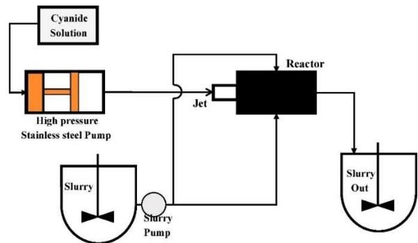
**Figure 7** Schematic diagram of the Jet reactor experimental setup.(Mbayo *et al.*, 2019)
