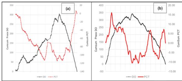
**Figure 2** Effect of pre-oxidation dissolved oxygen: (a) Period D – Oct 2015 to July 2016; (b) Period G – Jan to Dec 2018 on the concentrate leach solids residue (pumpcell circuit tails (PCT)).
