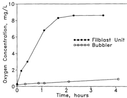
**Figure 6** DO Concentration in Pulp During Aeration Tests with Filblast Unit and Bubbler (Gas Flow Rate: 0.75 L/min)(Bodnaras *et al.*, 1993)
