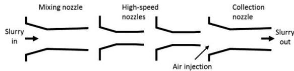
**Figure 8** Schematic of Mach reactor (Ross *et al.*, 2019).
