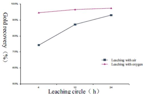
**Figure 4** Compared oxygen with air in bottle roll leaching (Zhongling *et al.*, 2015).
