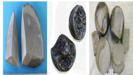
Figure 2. Examples of Premature failures of grinding balls
