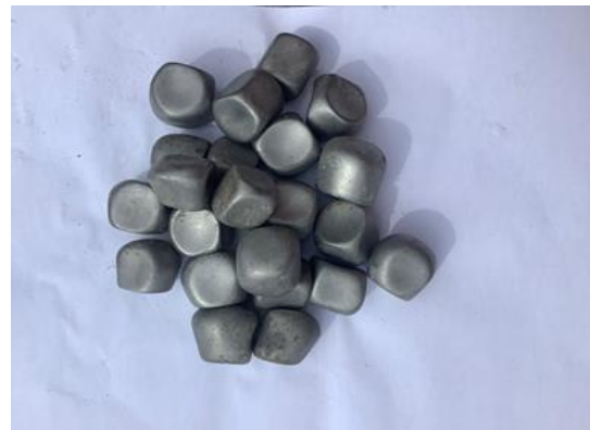
Figure 1b. Worn out balls from ball mill
