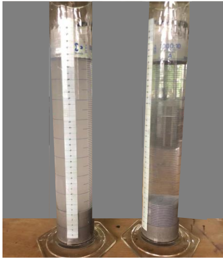
Figure 1 Settled Slurries in Setup A (conditioned with lime) and B (conditioned with Lime and 0.1% vol/vol Flocculant) from Mine 1
