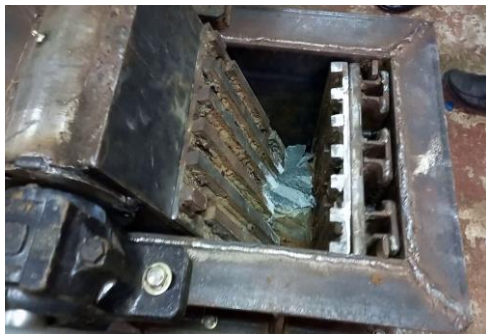
Figure 10 The New Jaw Crusher in Operation
