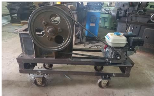
Figure 9 The Newly Manufactured Single Toggle Jaw Crusher
